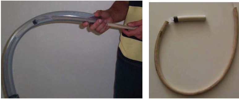
Fig. 25. Guidance control test in a colon-like tube
