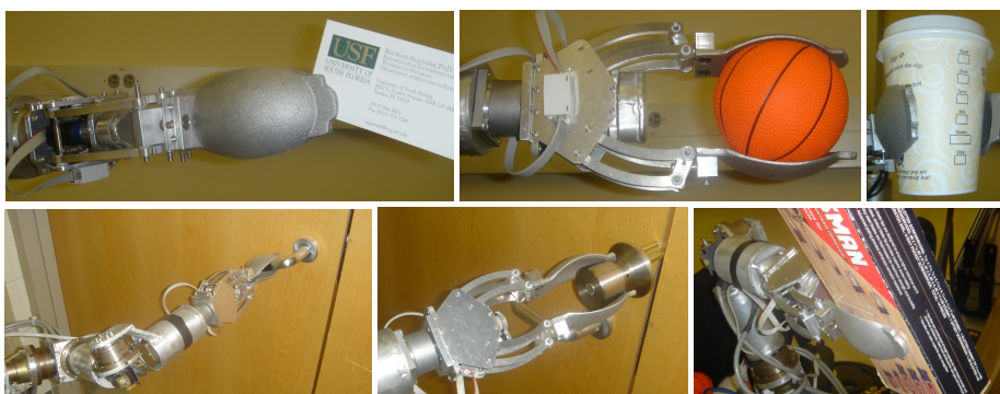
Fig. 12. Using the new gripper in typical ADL tasks.
