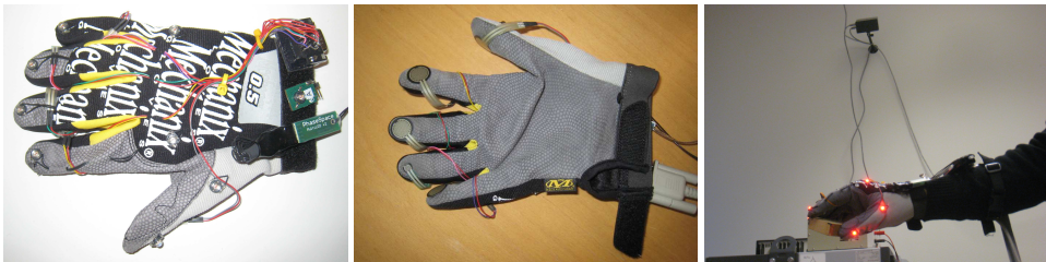
Fig. 8. Left: The glove used in the Impulse motion capturing system from PhaseSpace. The glove from the top showing the LEDs. Middle: The glove with the tactile sensors mounted on each finger tip. Right: The system in use showing one of the cameras and the LED on the glove.
